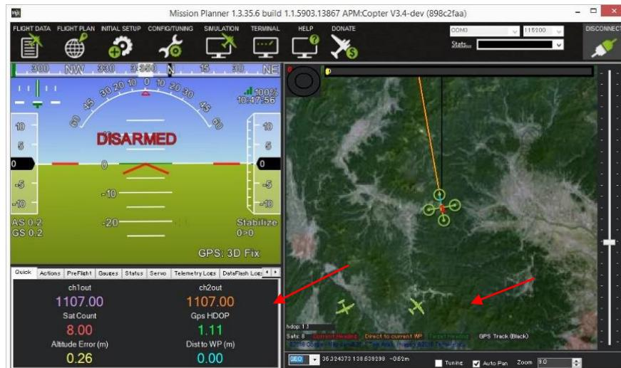
**Figure 12. Mission planer Provides information regarding the UAS Status and gathers flight data from ADS-B Equipped aircraft in the area**
