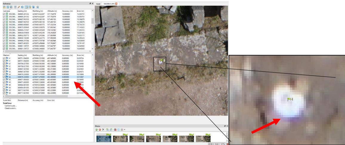
**Figure 17.** Control point (GCP) and its target.
