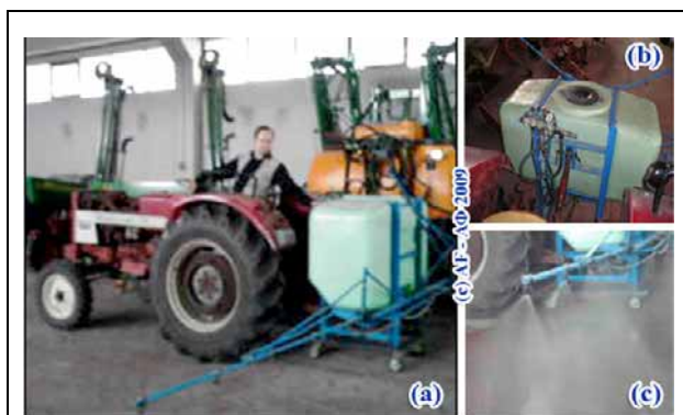
Fig. 1: a) The sprayer (boom) machine mounted on the tractor. b) Detail of the sprayer machine. c) Detail of the boom with the nozzles discharge.
