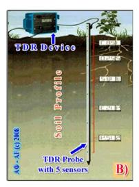
Figure 3. TDR device and probe with sensors.
