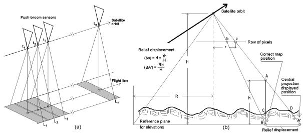
Figure 6. (a) Geometry of push-broom imagery, (b) The relief displacement in central projection.
