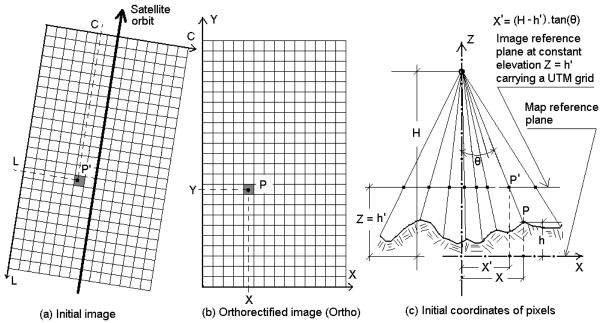
Figure 7. Original and orthorectified image with analysis of geometry for horizontal corrections when the elevation is known.
