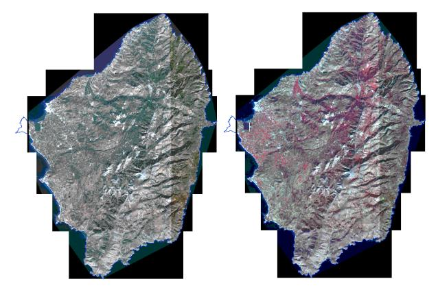
Figure 3. Left: The island of Naxos in R,G,B channels. Right: using channels IR, R, G. Satellite image of GeoEye-1 of 0.5 meter spatial resolution pan sharpened in four 11-bit channels dated October 23, 2009.
