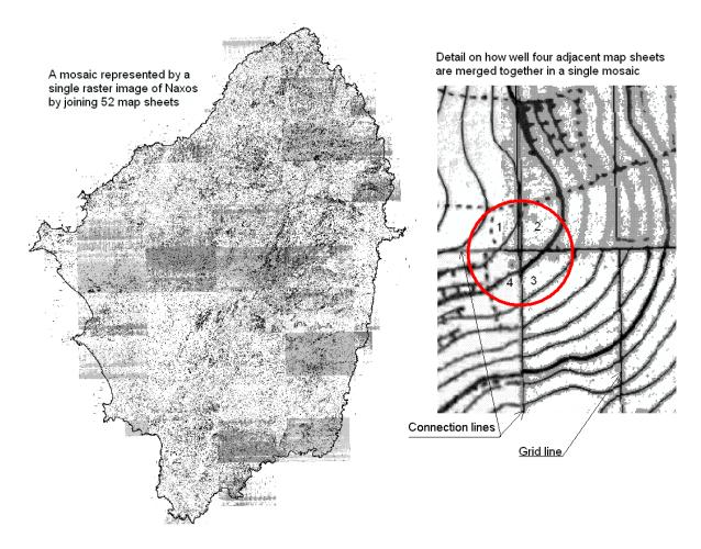
Figure 2. The mosaic of the 52 merged map sheets and a detail sowing the precision at the connections.
