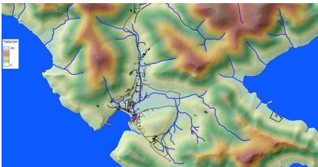
Fig. 7. The two watersheds that affect flooding in the settlement of Pserimos are visible in the relief form of the digital elevation model. Source: J. N. Hatzopoulos, Remote Sensing and GIS Laboratory.
