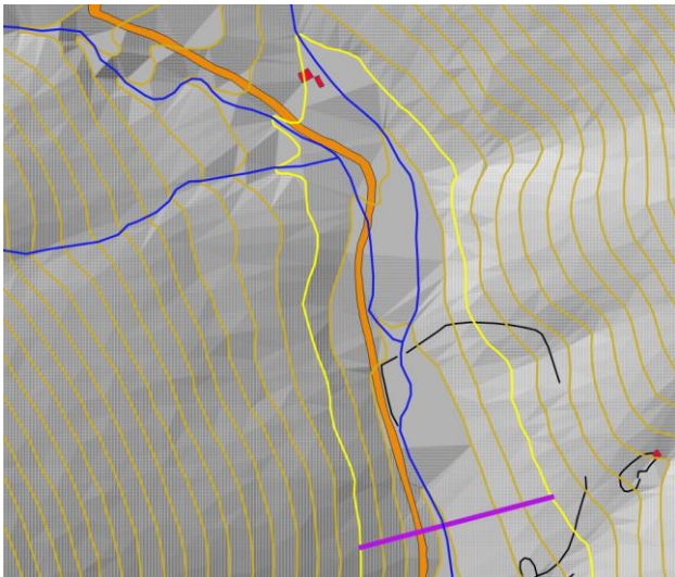
Figure 12. The proposed dam has a frontage of 120 meters and an area of 27000 m 2 . Source: I. N. Hatzopoulos Remote Sensing and GIS Laboratory.
