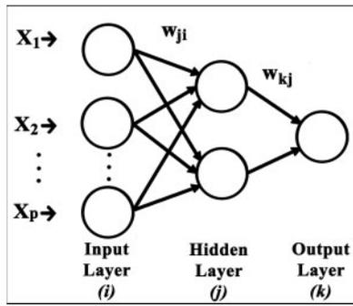
Fig. 8. Backpropagation neural network with one hidden layer and one output neuron.
