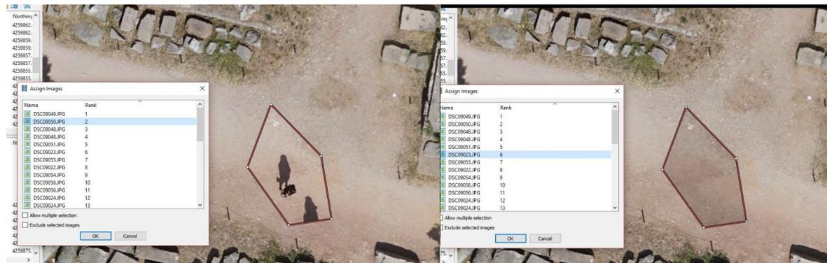
Figure 23. Manual image assignment to the orthomosaic process, to remove unwanted moving figures
