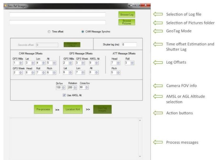
Figure 15. Mission Planner Geotagging tool interface
