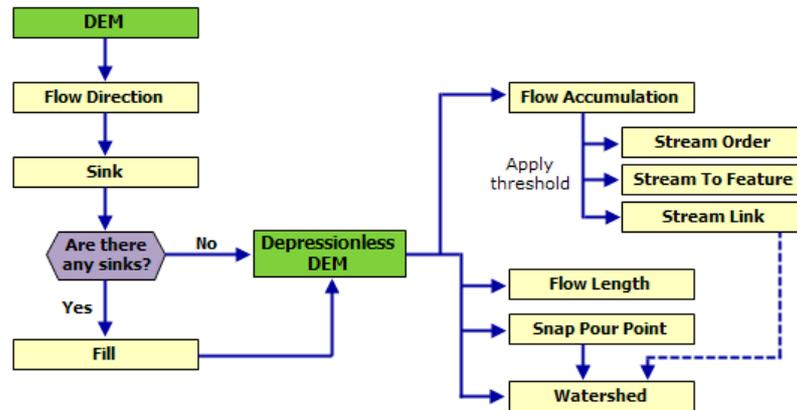
Figure 32. Hydrological modelling (Courtesy of ESRI ArcMap tools)
