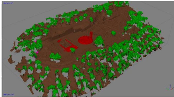
Figure 20. Classified Dense Cloud to: Ground, Vegetation and Structures
