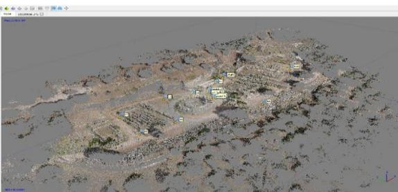
Figure 18. Sparse Point cloud generation and GCP'S (303.436 Points).
