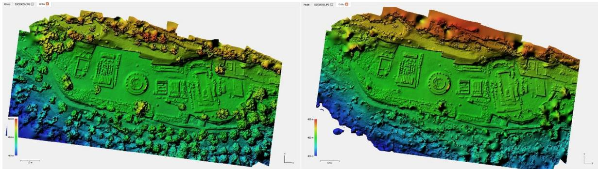
Figure 21. DEM Variants, with and without vegetation, respectively
