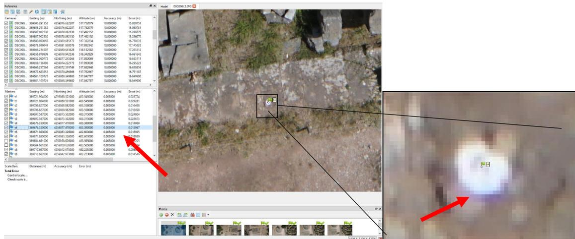
Figure 17. Control point (GCP) and its target.
