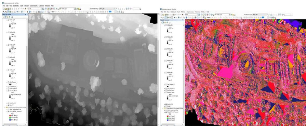
Figure 31. DEM of tholos in GIS Software and calculated Flow Direction
