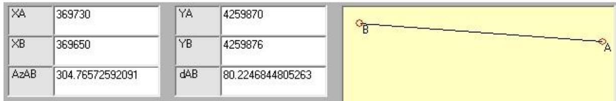
Figure 2. The output of the computation of azimuth and distance.
