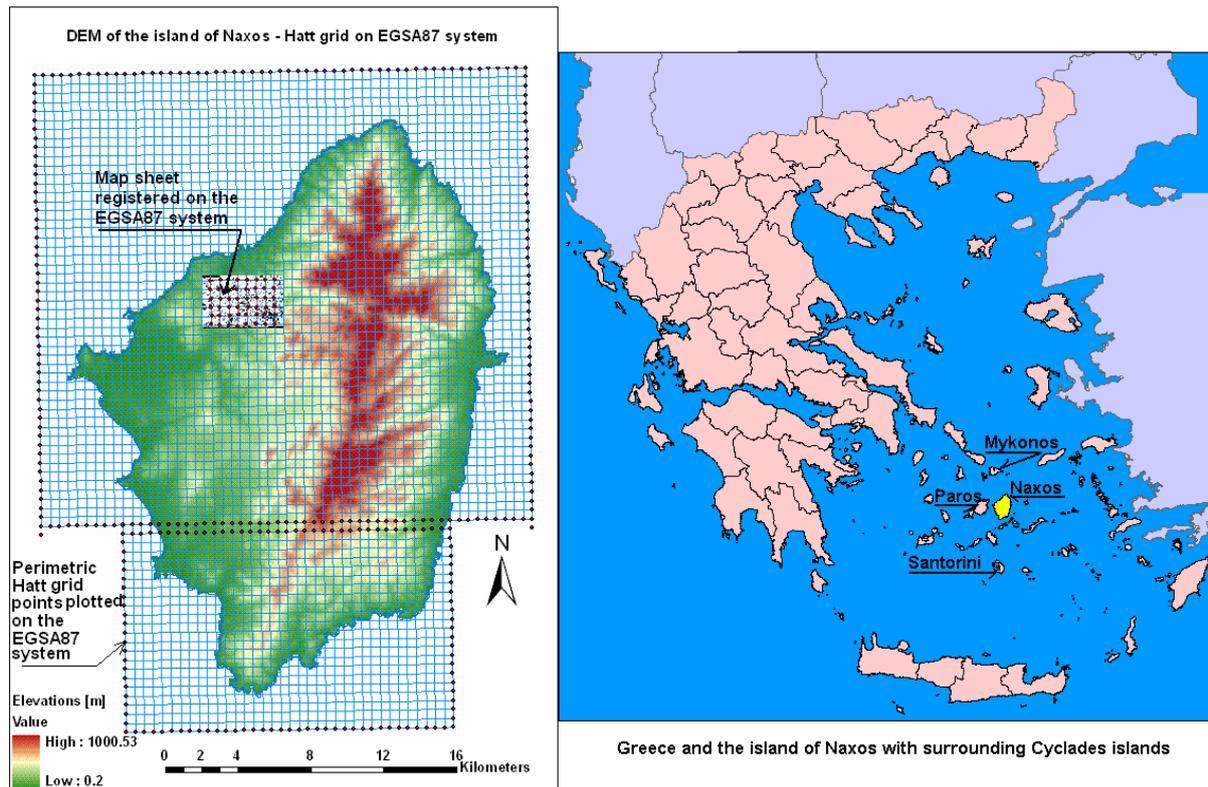
Figure 1. The Hatt grid on EGSA87 coordinate system helps to register all map sheets on this system.
