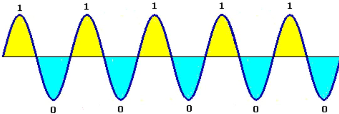
Figure 17. A pulse generated by the clock having a uniform code of: 1 0 1 0 1 0 1 0 ...
