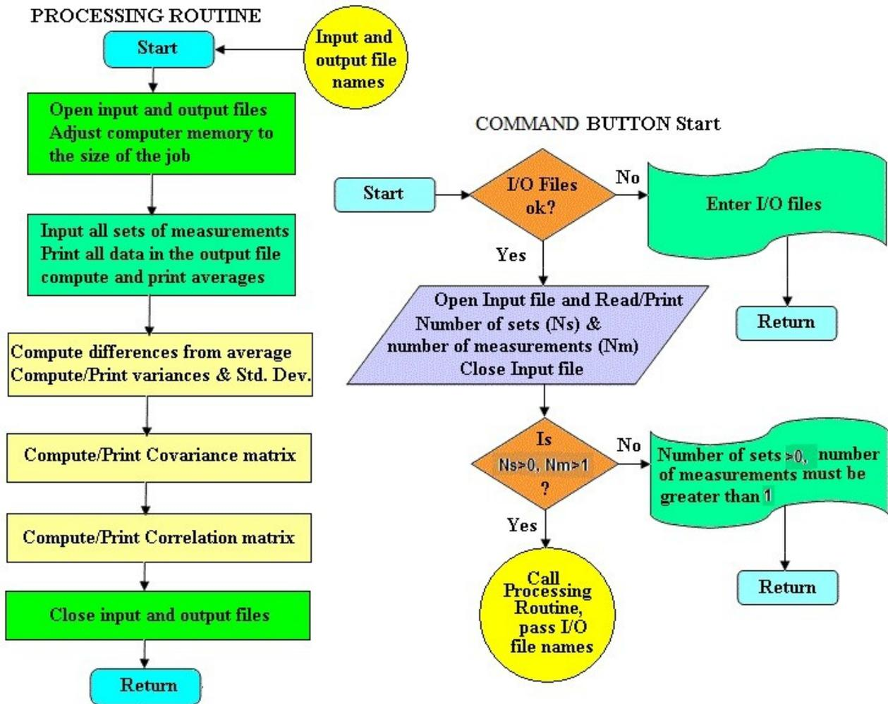
Figure 21. A flowchart of processing routine (left) and Command button “Start” (right).
