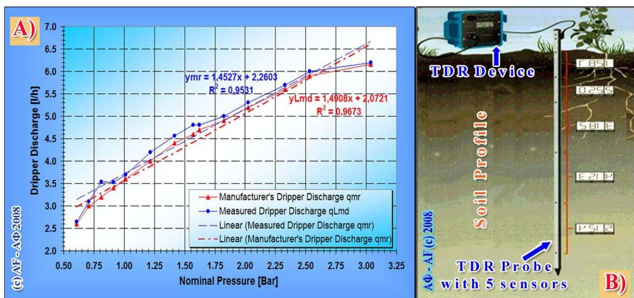
Figure 3. A) Diagram of dripper's discharge vs. nominal pressure from the manufacturer's measurements and from laboratorial measurements. B) TDR device and probe with five sensors.
