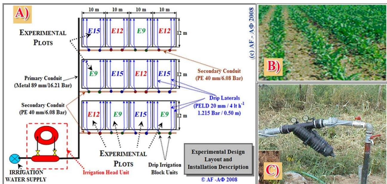
Figure 2. A) Layout of the experimental plots: Treatment E9, E12, E15 = irrigation session every 9, 12 and 15 days B) View of the maize's experimental field in the farm of TEI/L. C) View of the hydrocyclone filter.
