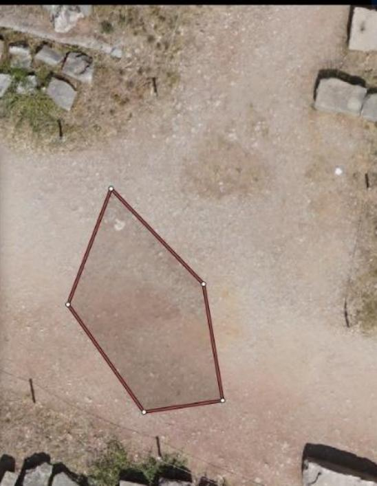
Manual image assignment to the orthomosaic process, to remove unwanted moving figures
