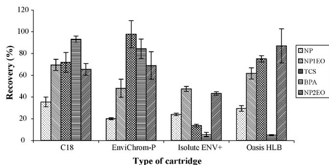
Fig. 2. Mean recoveries (%) of the target compounds in wastewater using different types of SPE cartridges.
