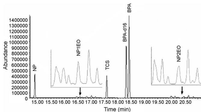
Fig. 1. Chromatogram of a standard solution containing  $1 \text{ mg l}^{-1}$  of the target compounds and the IS (BPA- $d_{16}$ ) in SIM mode.
